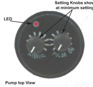
Setting Knobs shown at minimum settings between pulses. Times are from 5 seconds to 1 minute.
